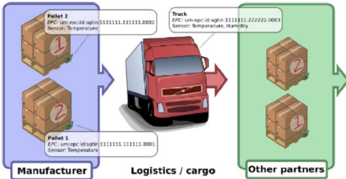
Fig. 2. Example Scenario for condition monitoring of refrigerated products in the Supply Chain
